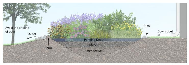
Figure 5: The layout of a rain garden should include both an inlet for runoff to enter the system and an outlet for water to exit. To protect against soil runoff, place a small berm prior to the outlet. The depression of the rain garden should be composed of amended soil and then a top layer of mulch.
