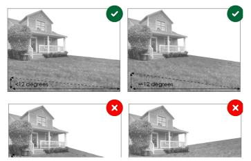
Figure 4: When placing a rain garden, ensure that the slope of the lawn is equal to or less than 12 percent.
