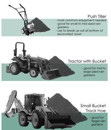
Figure 7: Excavation equipment should be chosen based of size of rain garden.
