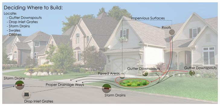
Figure 3: When determining where to build, consider the typical drainage patterns of your area, signified by the black lines above. If placed correctly, the runoff from your building will enter the rain garden system, depicted by the red lines.
