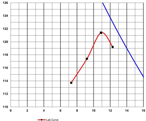
Maximum Dry Unit Weight & Optimum Water Content Zero Air Voids
