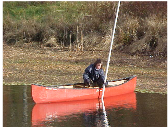
Figure M5.2: Measuring pond depth from canoe.
